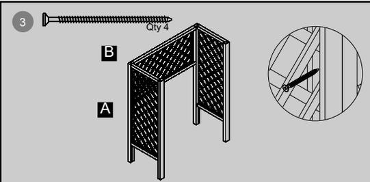
Fix the back panel to both of the side panels making sure that it is in line with the top. Fix this in place using 2 x 60mm screws for each side screwing through the groove in the panel.
