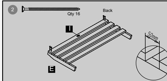
Place the long battens across the shorter battens to create the bench seat and back. Make sure that the battens for the bench are spaced 50mm apart. Fix each in place using 2x60mm screws for each end.
