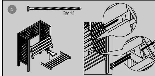
Place the bench seat between the two sides so that it is tight and the bottom of the bench is 378mm from the ground. Fix this in place using 2x60mm screws to fix each end to the posts of the sides sections.
