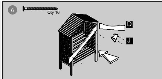
Place the barge boards to the roof so that the bottom of the curve is in line with the top of the roof and they meet at the apex. Fix each in place using 3x40mm screws.
